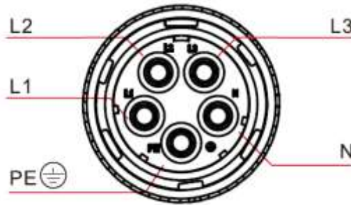
Figure 7.14.3 Internal structure of AC connector
