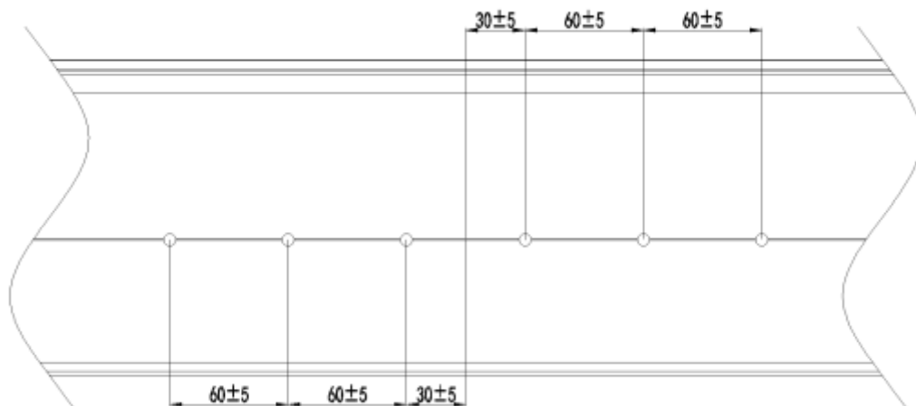
Figure 5.2 Position of Self-tapping Screw
