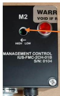
M2 High-Low Adjustment Screw
