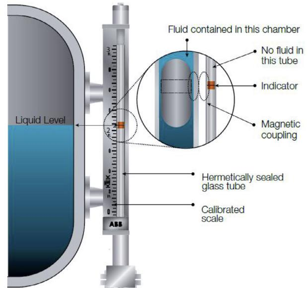
Figure 3 Magnetic Level Gauge Principle
