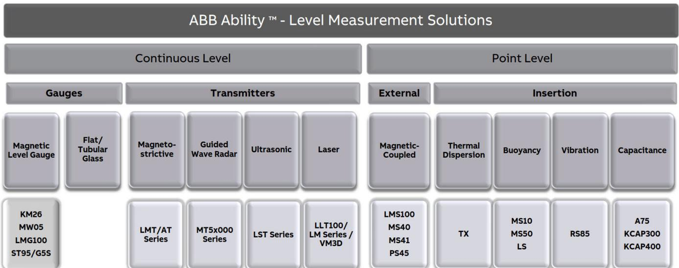
Figure 2 Level Measurement Solutions
