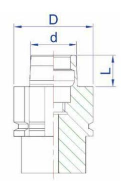
On equal external diameter of the flange (D), for forms A - C - E the larger taper diameter (d) is one size bigger than the other.
