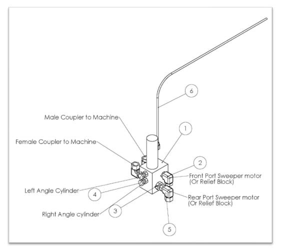
Angle Broom Valve Block Assembly – Detailed Parts List B
