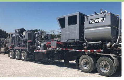
The Trican-designed Twin Cementer provides fully redundant systems to ensure the cement job can be completed under nearly any circumstance
