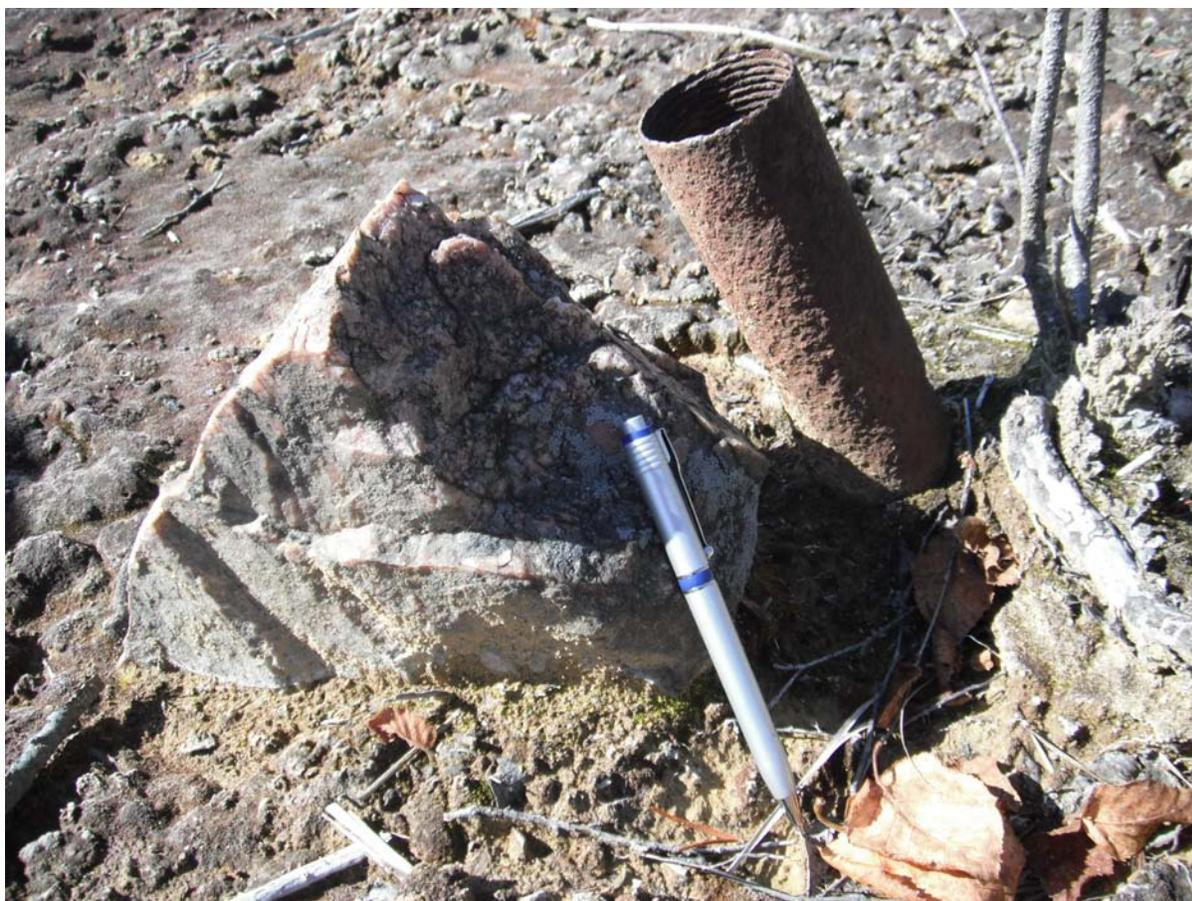
**Photo 3: Historical diamond drill hole casing at 460757E, 5181945N (Azm = 351°, Dip = -66°).**
