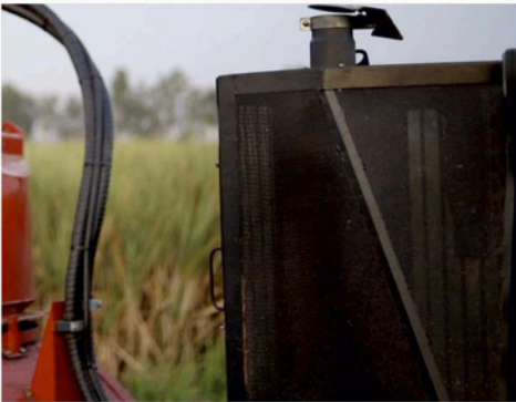
Improved Bird Cage Sealing Engine safeguarded from trash entry, improved productivity & safety
