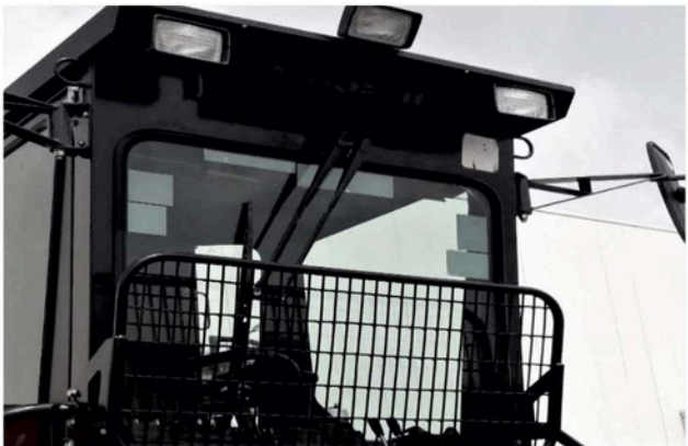
Cabin Windshield Guard Effective protection of cabin windshield from cane hits
