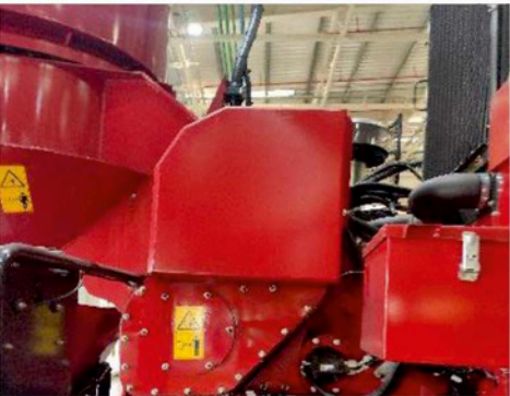
Chopper Flywheel Cover Additional protection for chopper flywheel
