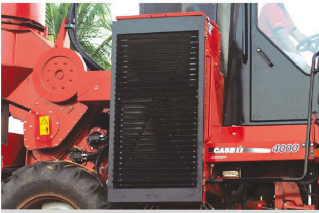
Bigger Radiator Increased cooling efficiency
