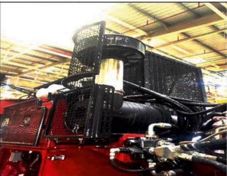
Pre Cleaner Protection guard Additional safety against cane hitting
