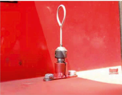
Relocated Dip Stick Ease of access & frequent opening of bird cage avoided
