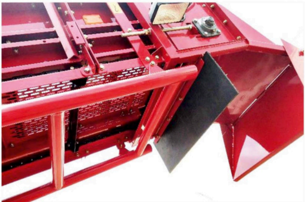
Elevator Rubber Flap Avoids the billets from falling onto the ground during Infilder filling
