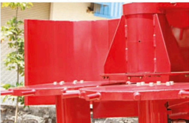
Disc-O-Gather Topper* Ensures excellent removal of Tops resulting in less trash going into machine & reduced fuel consumption
