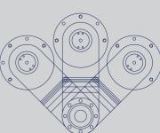
The Baudouin SCR catalyst adapts to any vessel layout. The system can rotate 360° on its axis to allow maximum mounting flexibility. In addition, the catalyst is 1m³ in volume, one of the smallest available on the market.
