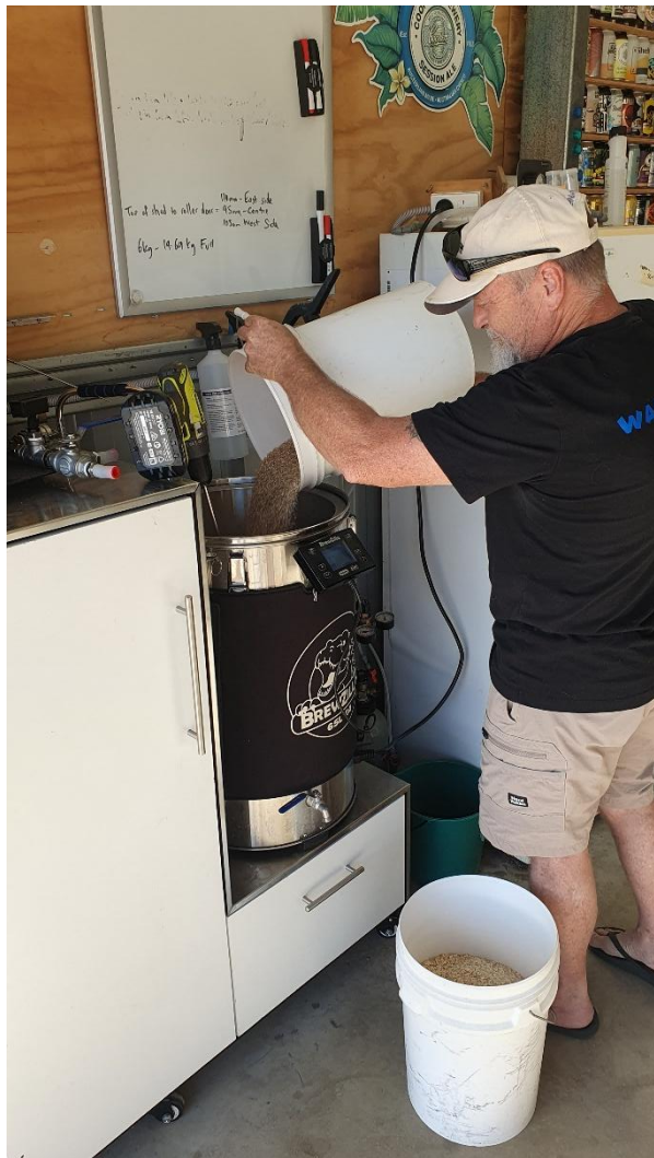
Milled grains going into the mash tun
