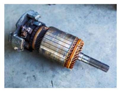
HERE YOU'LL SEE THE COMMUTATOR AND BRUSHES ASSEMBLY, LOOKING MORE CORRODED THAN THEY SHOULD.
