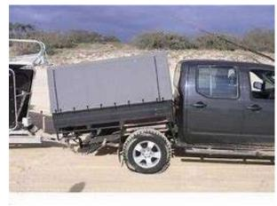
The problems come when drivers start adding custom trays, canopies, and heavy weights to that rear overhang, compounding the stresses on the chassis point between the cabin and tray. These stress limits can be exceeded when the ute and caravan / trailer in tow, go over undulating ground and the result can be a cracked chassis and a banana shaped chassis ute.
