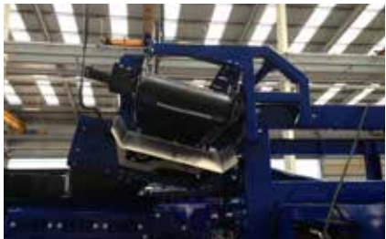
Overband Magnet- fitted to collection conveyor to extract ferrous metal.
