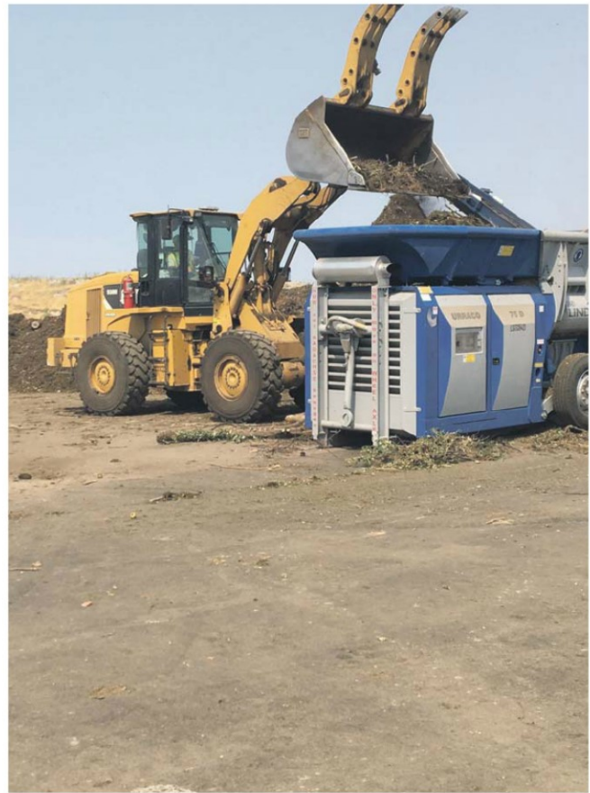
The Salt Lake County plant takes in approximately 44,000 tons of green waste every year, and the Lindner Urraco 75D mobile shredder is able to process up to 40,000 tons per hour.
