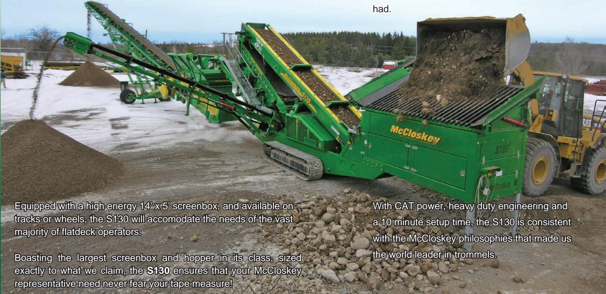
Equipped with a high energy 14' x 5' screenbox, and available on tracks or wheels, the S130 will accommodate the needs of the vast majority of flatdeck operators.
