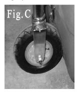
body or look for "forward" sticker on fork (see Fig. C left) Tighten clamp secure upper "T" bar. Tighten clamp with enclosed allen wrench so that upper "T" bar is secure and unable to be turned separately from lower fork, Fig. D.
