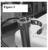
ening the screw may cause the upper "T" bar to stick.) When the cam arm is closed, the arm of the cam should point forward. Adjust the upper "T" bar to the desired height. Close the arm of the cam to lock the upper "T" in place. If the tension of the cam is too loose or too tight, the arm will not close. Adjust the tension on the cam via the nut opposite the arm cam. Square the upper "T" bar with the bottom fork. Tighten the lower clamp with a hex key from your tool pouch. Figure I
