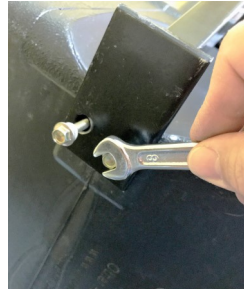
Front Mount Assembly On Bottom of Cooler
