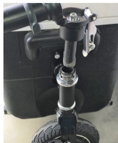
Insert Steering Neck into Wheel Assembly
