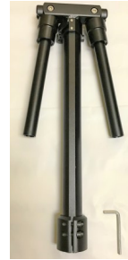
Steering Assembly with Neck Collar
