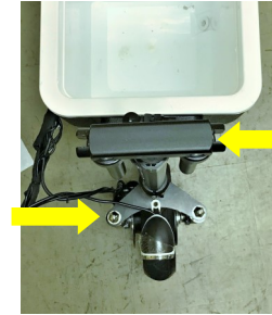
Steering Assembly aligned with Neck
