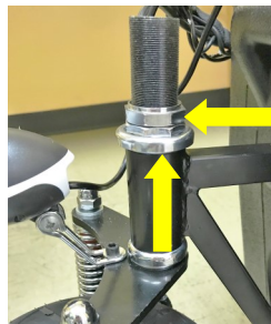
Top Steering Nut(left arrow), Steering Nut with Bowl(up arrow)
