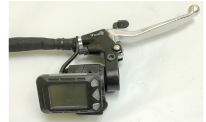
Throttle with Display, Right Brake Lever
