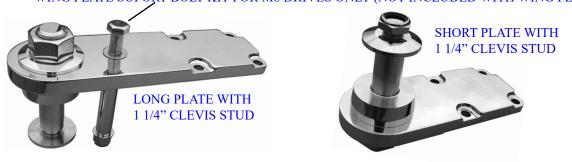
TB-71 TIE BAR KIT FOR MERC M6, M8 DRIVES 4 3/4" DROP TO CENTER DRIVE 24" MAX DRIVE CENTERS
