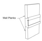
Predrill and countersink holes for flat head screws in the insert channel of the Mounting Rail.
