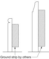
Trim the ends of the base molding as necessary and fasten the base molding to the "ground strip" already installed on the wall.
