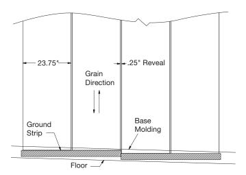
Establish a level line along the wall near the floor as a base for the wall panels. This line should be 1/2" lower than the finished height (either 4" or 6") of the base molding you are using.
