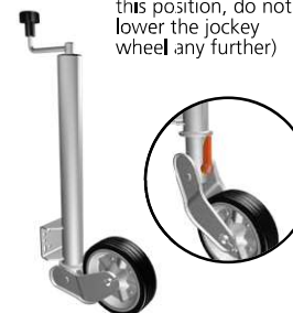
Automatic jockey wheel (rough adjustment using the flap mechanism and spindle drive)
