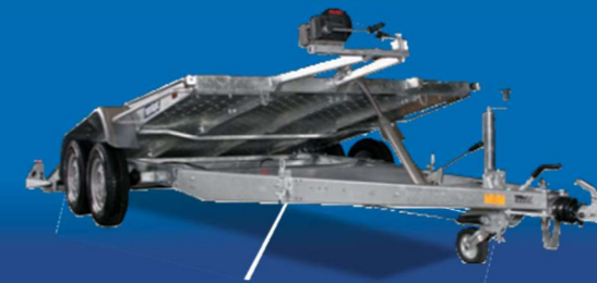
STANDARD ACCESSORIES Steel floor with raised holes. Strong and non-slip.
