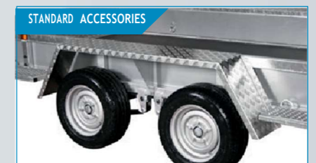
Powerful wheel fender in aluminum. Robust, non-slip and smooth.
