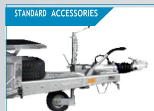
Powerful jockey wheel. 3.500 kg extra strong. Coupling w/lock on 3.500 kg models.
