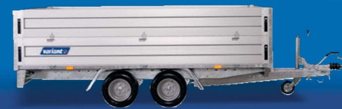
Dropsides: Increases the volume of trailers. Foldable and removable. Height 35 cm.
