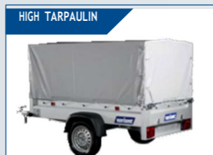
HIGH TARPAULIN Strong quality with opening in the sides and back. Inside height 105 cm when mounted.
