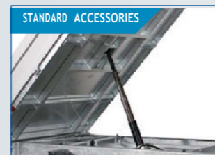
4-step piston, provides high tip angle, so gravel etc. easily slides off.
