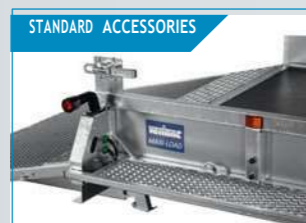
Non-slip pedestals all around and external lashing eyes.
