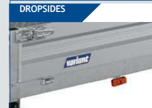
Aluminum, 35 cm. With hinges. Openable and removable.
