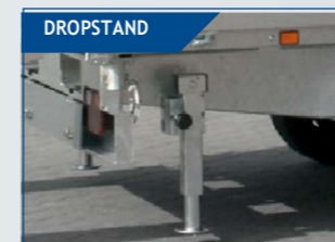
DROPSTAND Powerful and rotatable, provide secure and stable loading and unloading. Incl. hand crank for maneuvering.
