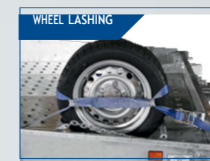
WHEEL LASHING Can be used with stop blocks as shown in the picture.
