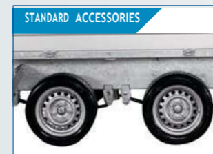
Leaf springs provide perfect suspension. 13" compact wheels provide low loading height.
