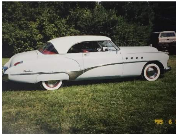
1949 Buick Roadmaster Riviera. This was the first true hardtop car ever produced.
