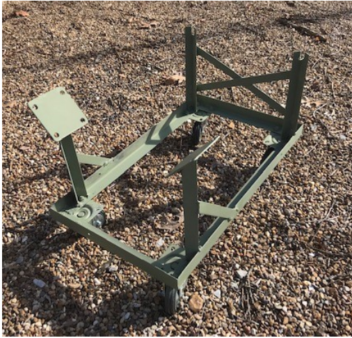
Front angle pads to mount to the engine mount pads on the block
