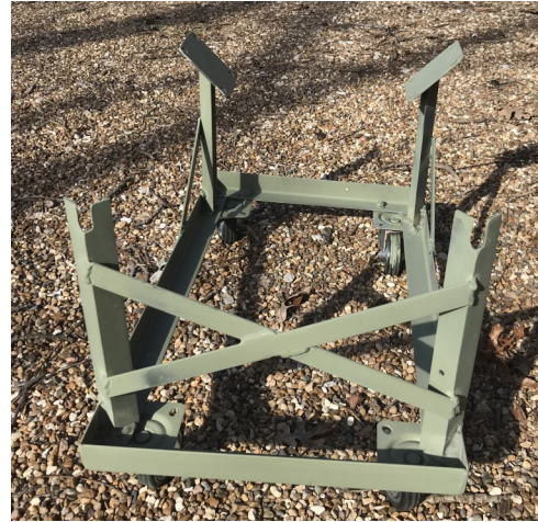
Rear of dolly showing the notches where the bolts in the bell housing sit. Also note the cross bracing.
