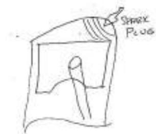
As the spark plug fires, the fuel and air mixture at the spark plug begins to burn. The burn then travels across the chamber in a controlled manner until all the fuel is burned, the resulting increase in pressure creates the force to push the piston down on the crankshaft and create power.
