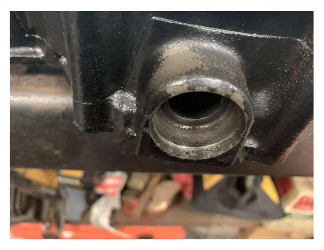
Don't get too aggressive, but lightly hitting the bore with a fine grit of emery cloth will clean up what little deposits remain. Now that the bore is cleaned up, wipe it down with your favorite solvent to remove any dust from the brushing and/or sanding process. Put a *LIGHT* coat of black RTV inside the bore, similarly coat the snout on the coolant manifold and the O-ring and put it together.
