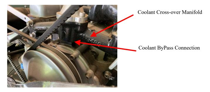
The above photograph shows the coolant cross-over manifold and the bypass connection. Unlike most engines, the coolant from the cylinder heads goes into this crossover manifold and into the thermostat housing. At the base of the manifold is a cast nipple that fits inside a bore in the front cover.
