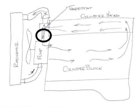
We see circled the bypass line. As the engine is not up to normal operating temperature, and the thermostat is closed, coolant flows through the bypass line and back to the suction side of the water pump. Flow through the block and head are subsequently maintained to prevent localized heating and boiling.
