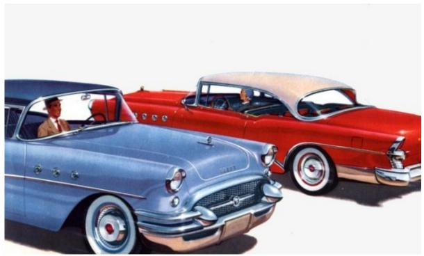
So began the custom of three holes per side on lesser Buick models and four per side on the top-of-the line offerings, with slight tweaks from year to year. In the 1955 lineup (above) the Special (264 CID V8) featured three mouseholes in each front fender, while the Century, Super, and Roadmaster (322 CID V8) boasted four per side.
