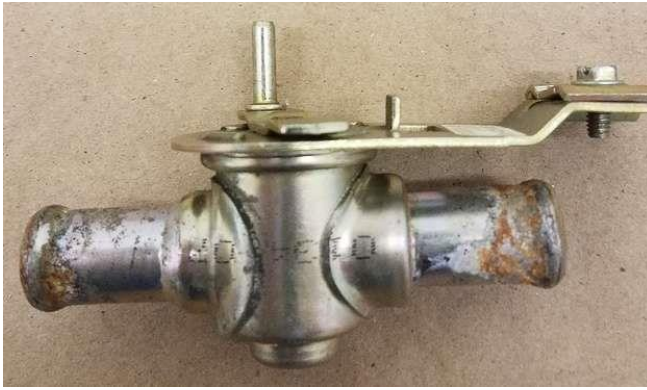
Old Heater Shut-off valve
