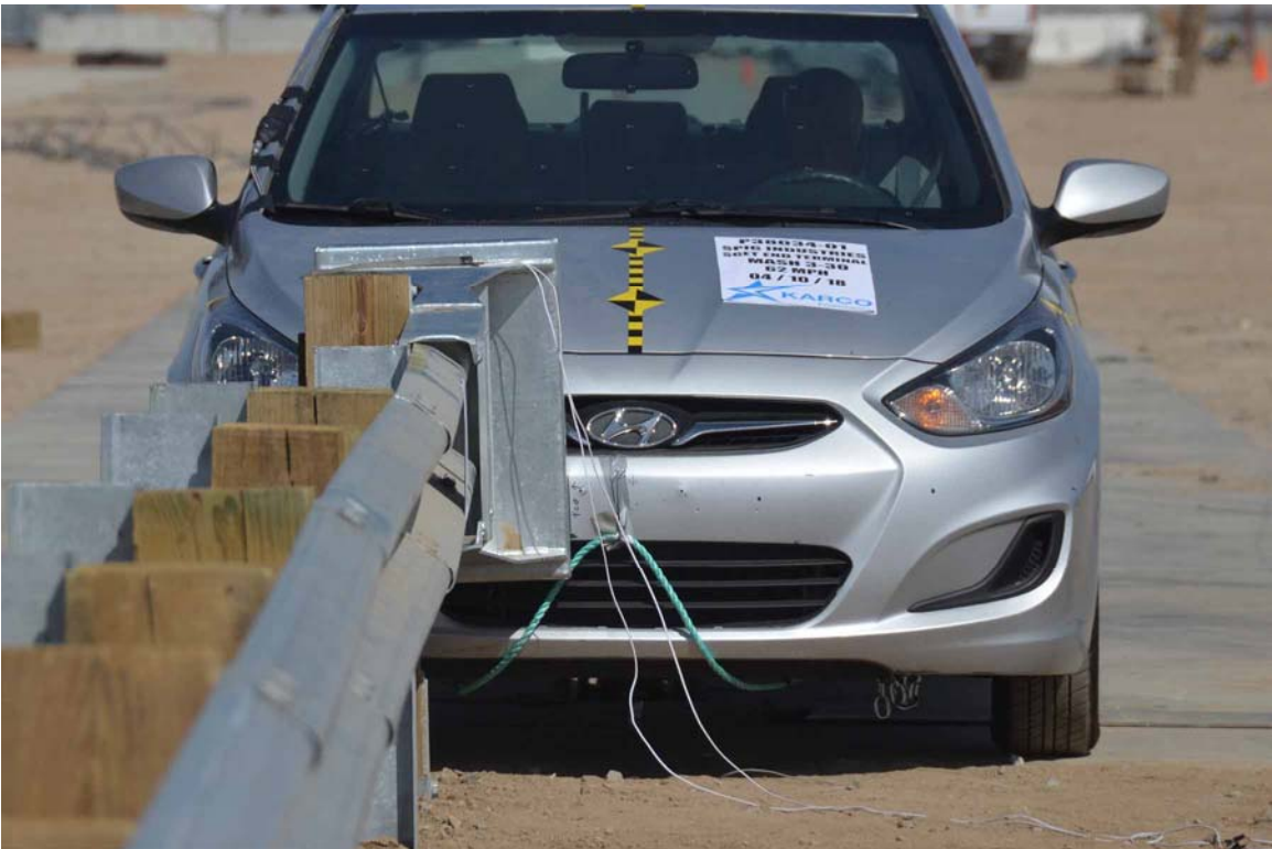
FIGURE 6. Test Setup, Close-Up
