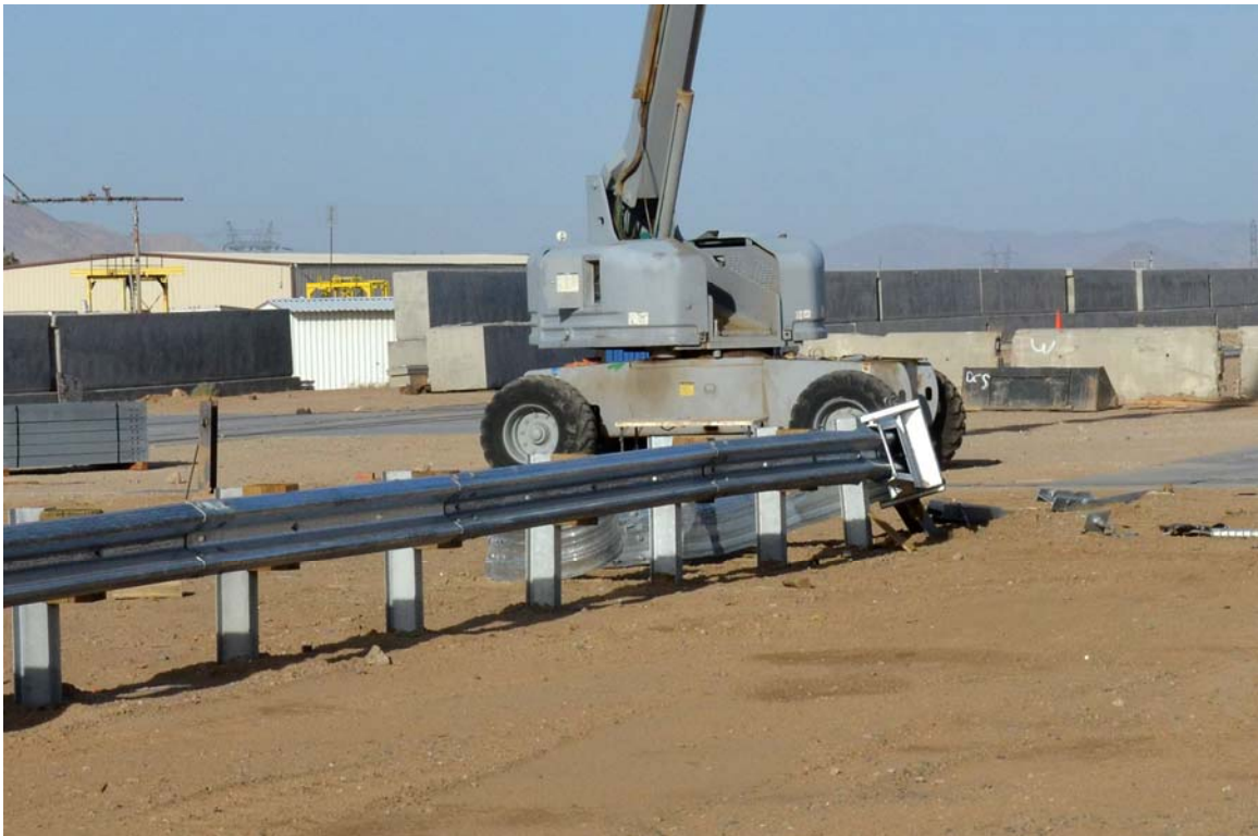
FIGURE 22. Post-Test Right Rear \frac{3}{4} View of Test Article
