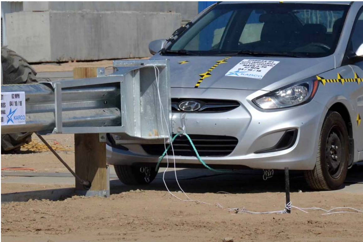
FIGURE 4. Test Setup, Close-Up
