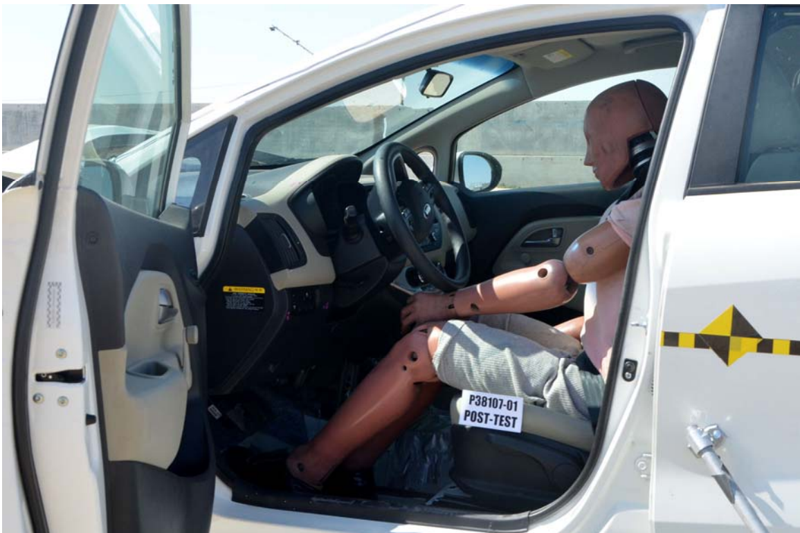
FIGURE 50. Post-Test Driver Side Occupant Compartment
