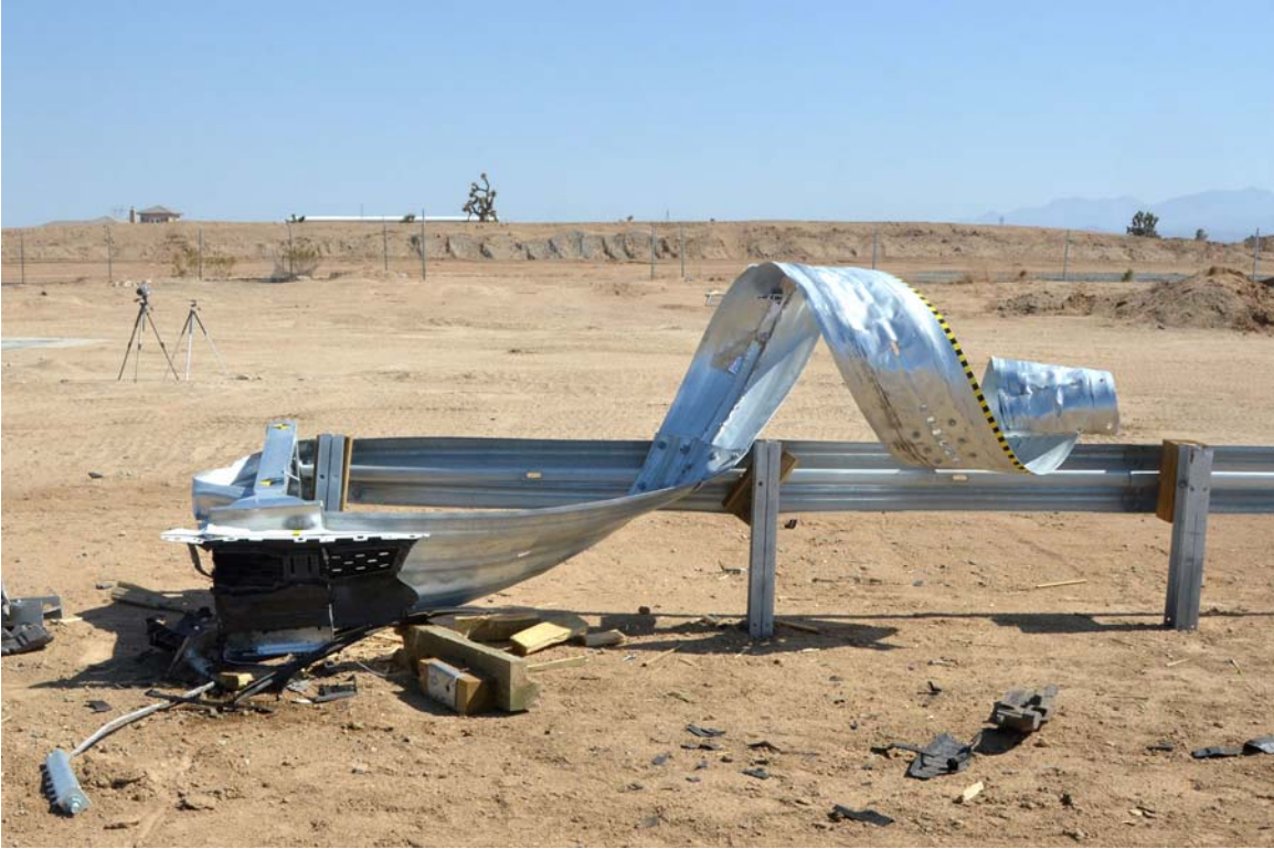
FIGURE 31. Test Article Damage
