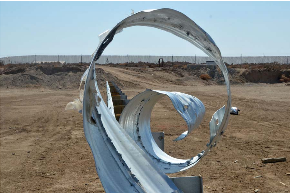
FIGURE 34. Test Article Damage
