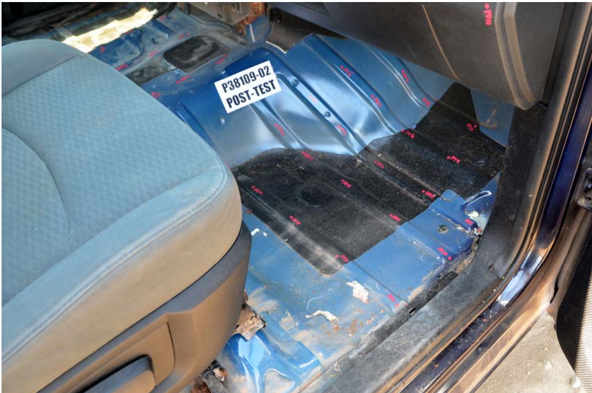
FIGURE 56. Post-Test Passenger Side Floorpan
