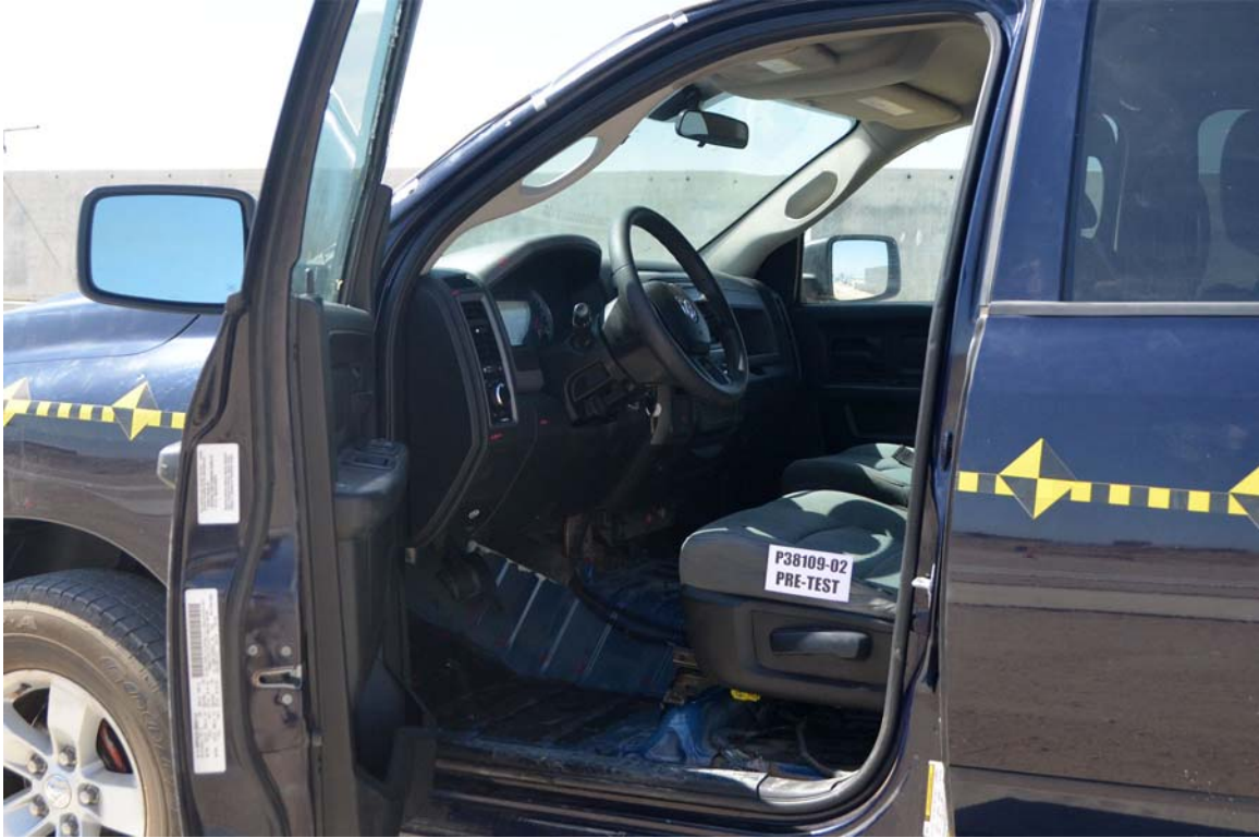
FIGURE 49. Pre-Test Driver Side Occupant Compartment
