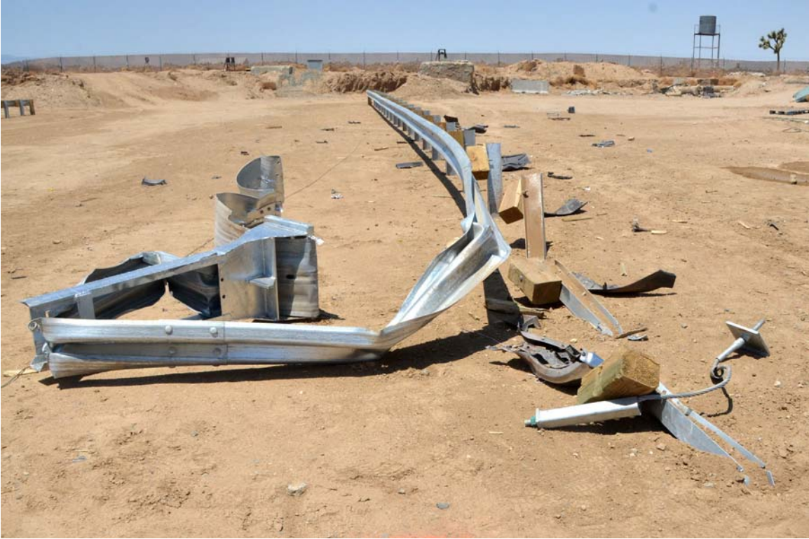
FIGURE 31. Test Article Damage
