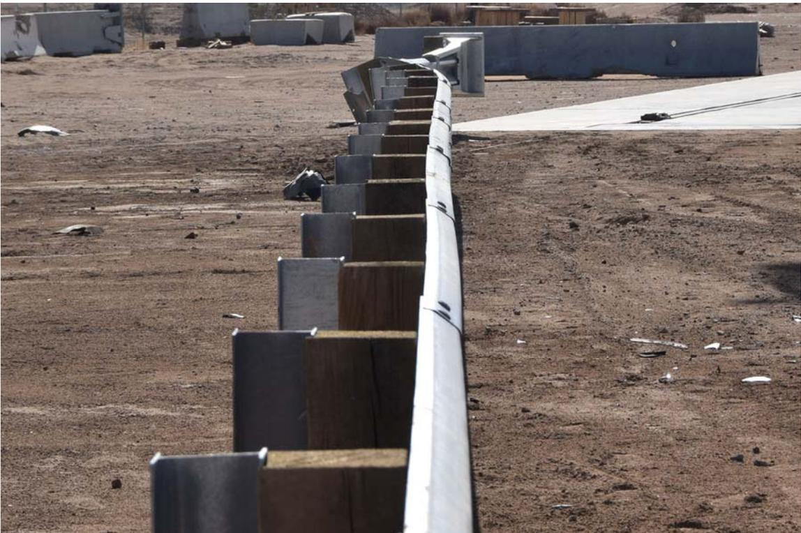
FIGURE 24. Post-Test Rear View of Test Article
