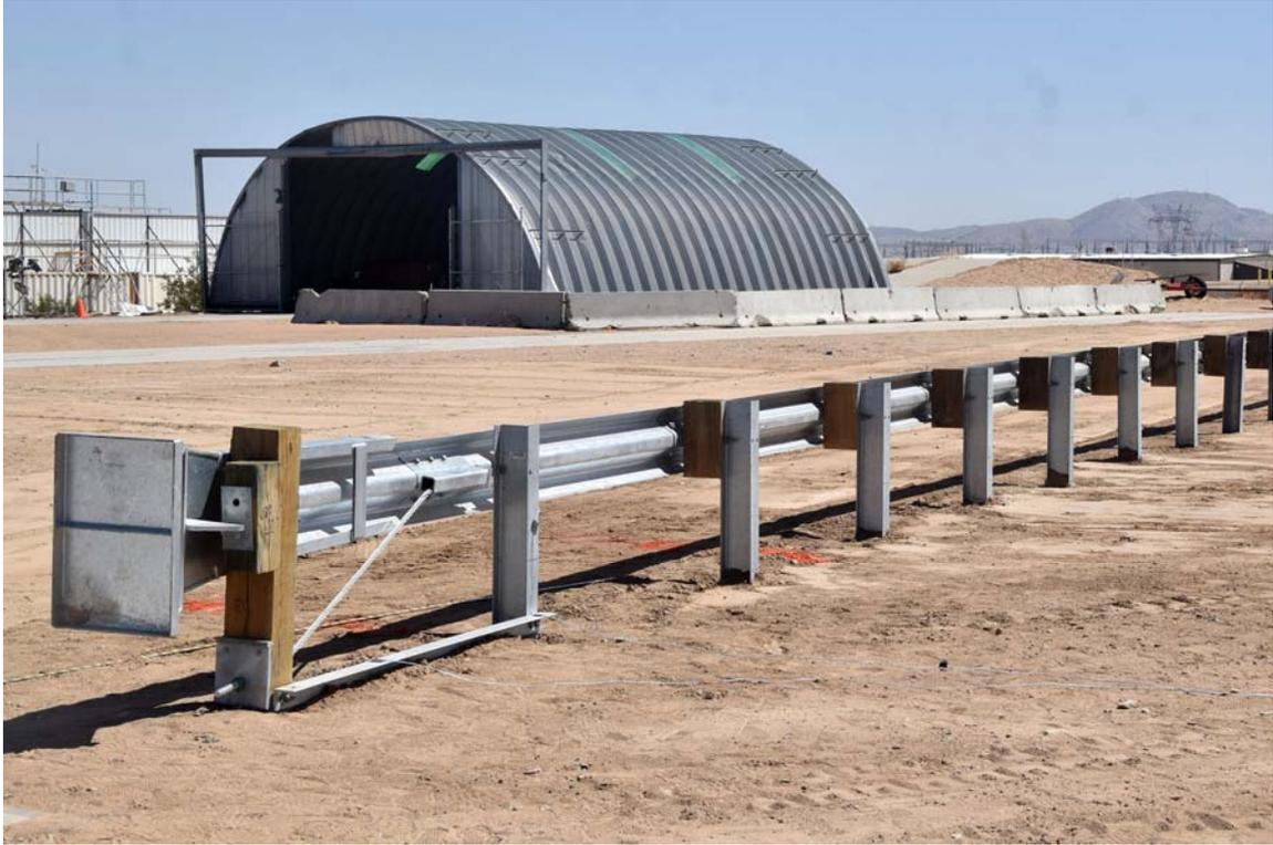
FIGURE 29. Pre-Test Left Front  $\frac{3}{4}$  View of Test Article
