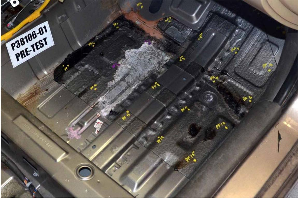
FIGURE 55. Pre-Test Passenger Side Floorpan
