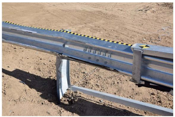
FIGURE 33. Test Article Damage
