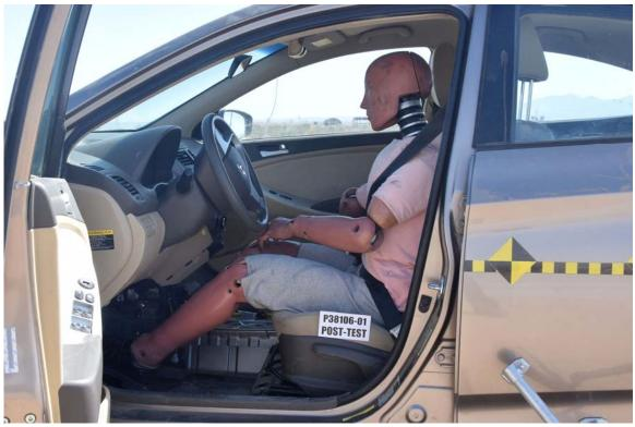
FIGURE 50. Post-Test Driver Side Occupant Compartment
