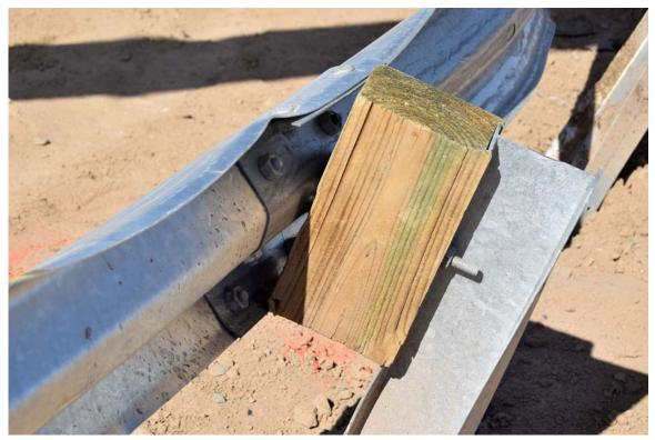
FIGURE 36. Test Article Damage
