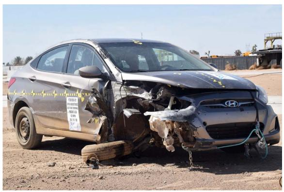
FIGURE 44. Post-Test Right Front 3/4 View of Test Vehicle
