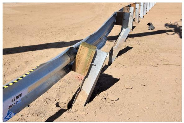
FIGURE 35. Test Article Damage
