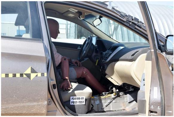
FIGURE 54. Post-Test Passenger Side Occupant Compartment
