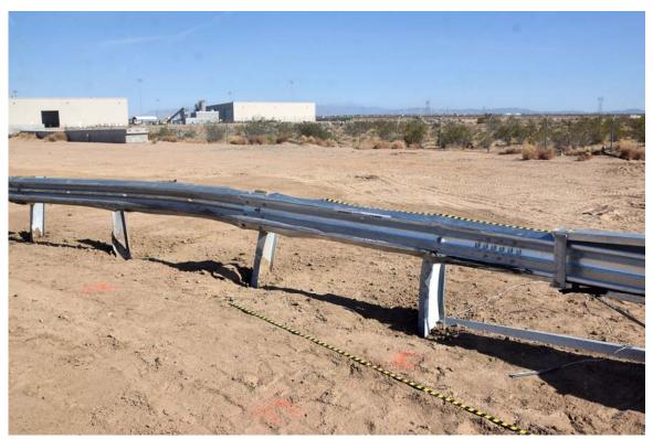
FIGURE 32. Test Article Damage
