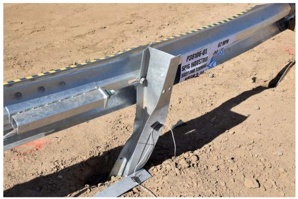
FIGURE 34. Test Article Damage
