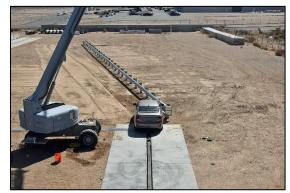
TESTED TO: Manual for Assessing Safety Hardware (MASH 2016) Test 3-34
