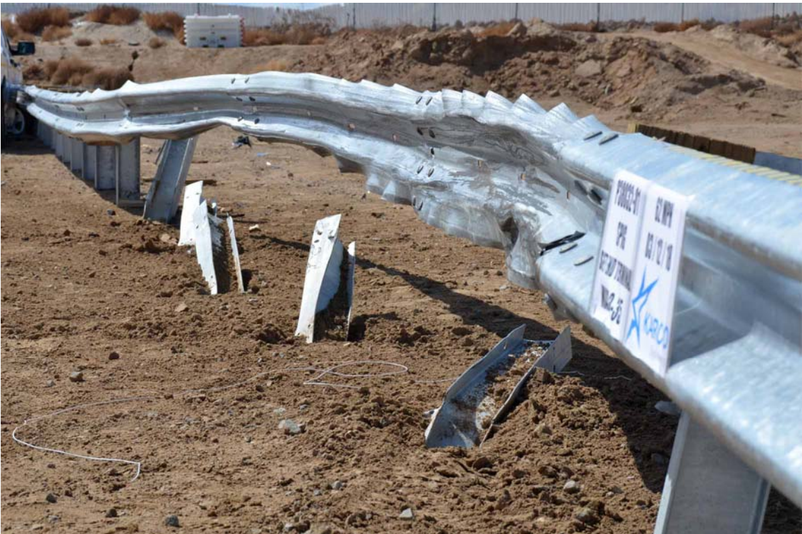
FIGURE 32. Test Article Damage
