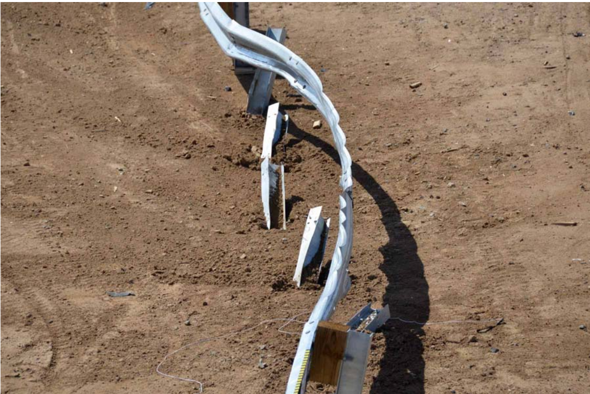
FIGURE 34. Test Article Damage
