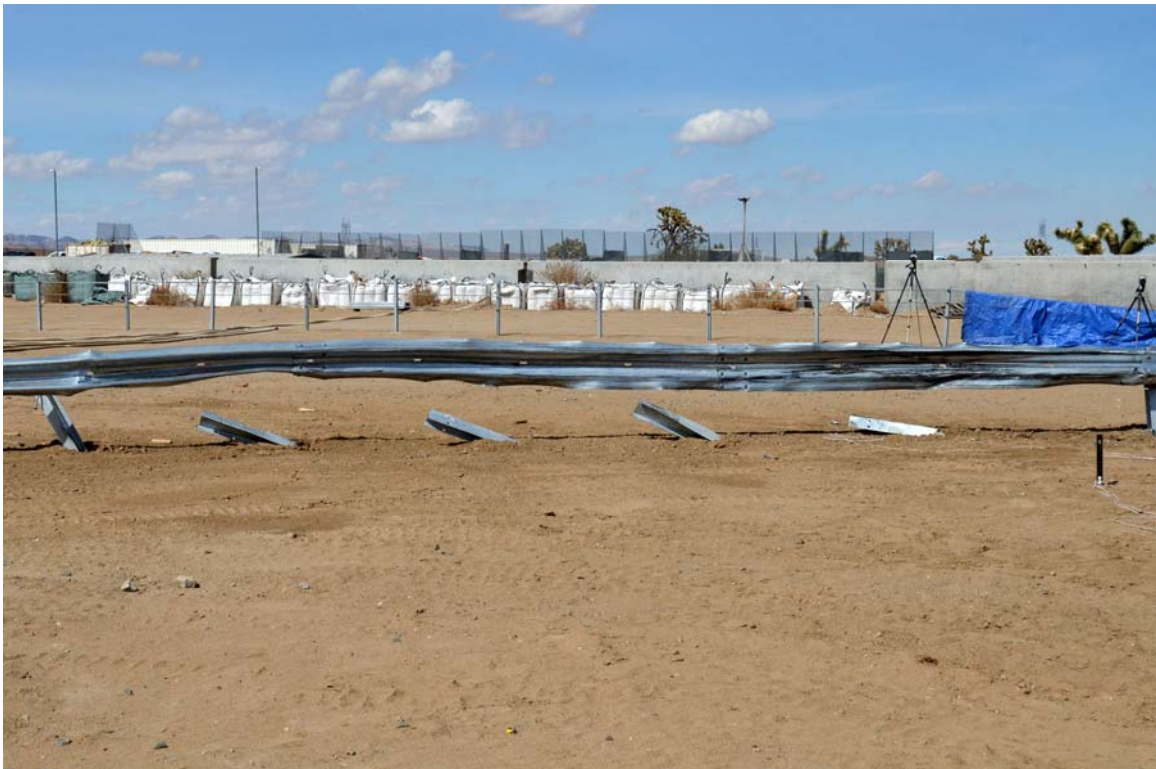
FIGURE 34. Test Article Damage
