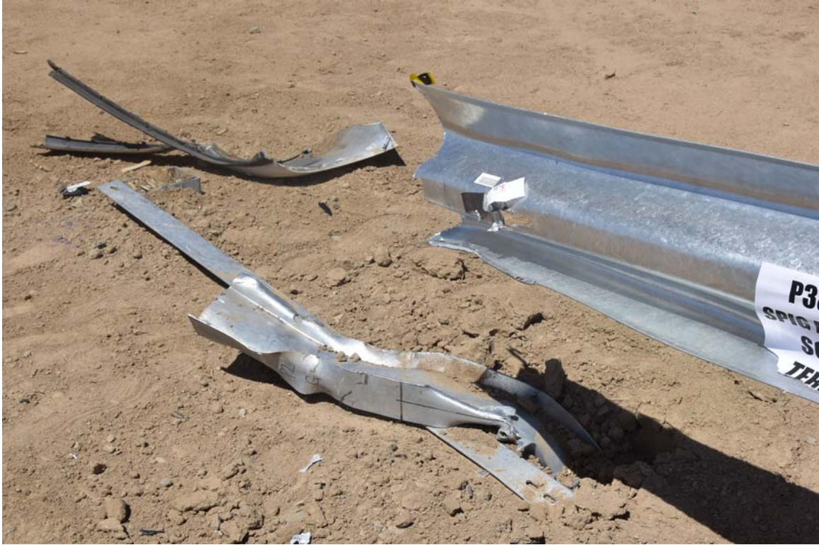
FIGURE 33. Test Article Damage
