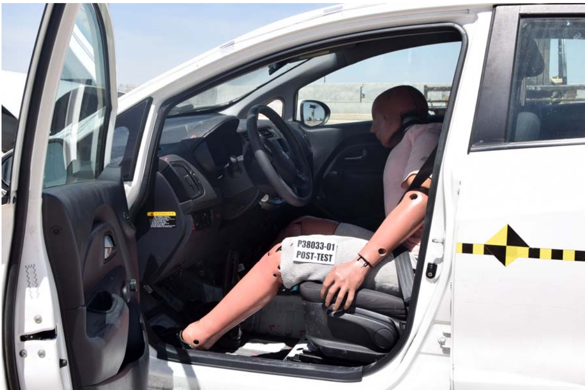
FIGURE 50. Post-Test Driver Side Occupant Compartment
