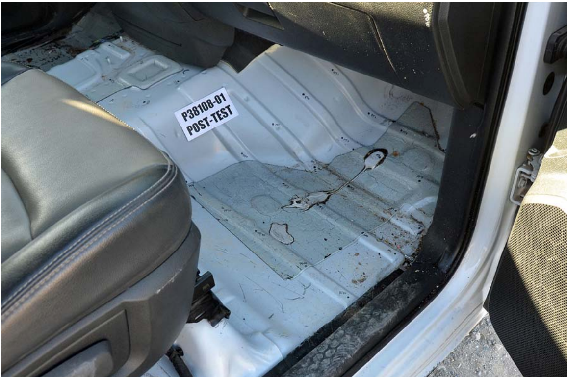
FIGURE 56. Post-Test Passenger Side Floorpan
