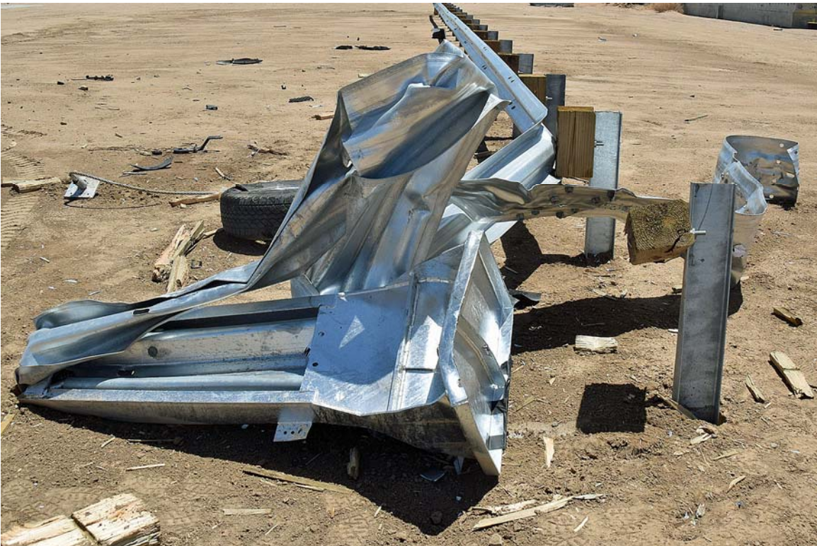
FIGURE 34. Test Article Damage
