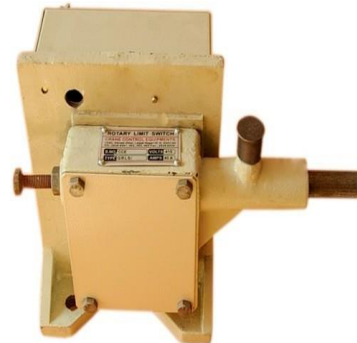
Rotary Geared Limit Switch
