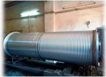
Seamless Pipe Rope Drum
