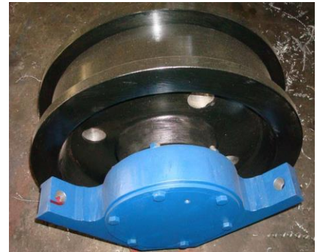
Wheel & Wheel Assembly & L block
