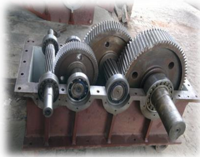
Gear Box internals
