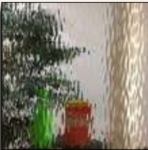
Water Privacy rating: 5
