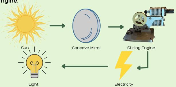
The engine makes electricity from the heat. Electricity turns the LED lamp ON.
