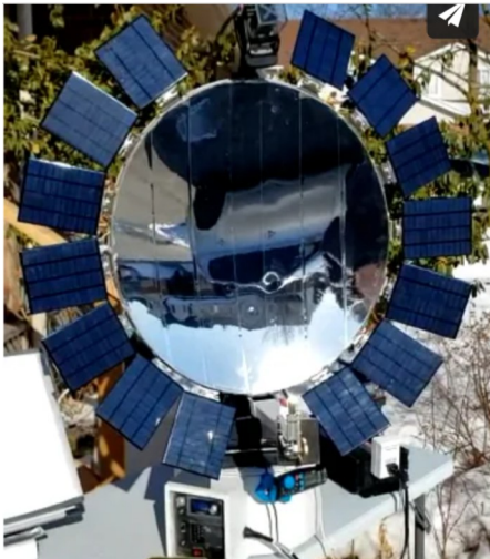
Automatic sun tracking dish with Stirling engine – GREENBMG INC.
