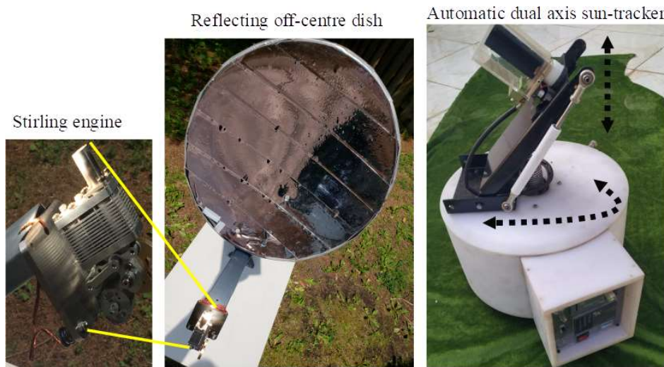
Automatic sun tracking dish with Stirling engine – GREENBMG INC.
