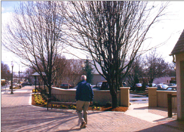
The photo above shows a 30" wall used to screen a parking area from the sidewalk. The hedge or wall, plus trees, is accommodated by the required 5' setback.
