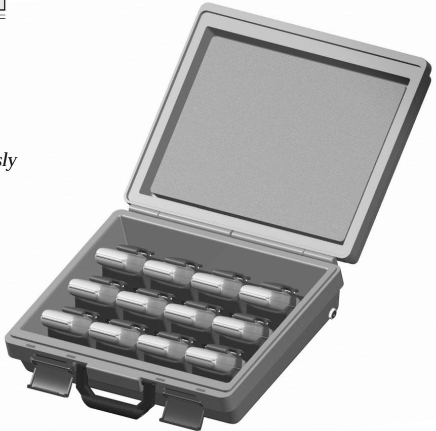
**T**he NBC 9-3-12 Digital Fast Charger is designed to simultaneously charge and store up to twelve COMTEK 216 or 75 series receivers and/or transmitters. The charger will charge 3 volt (two AA size batteries) or 9 volt nickel-metal hydride (Ni-MH) batteries. The charger will automatically select the charging mode for the type of battery being used. It is also equipped with a self-diagnostic capability to identify faulty batteries and to ensure safe operation.
