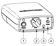
**4** ON / OFF SWITCH: This switch turns the receiver on and off.
