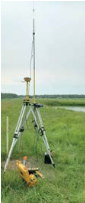
RTK Base Station
